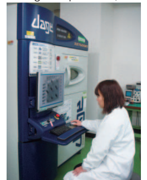
Analyzing electronic component quality by soft X-ray
