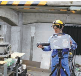
Vacuum arc observation experiment for VCB development
