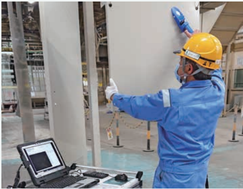
Surface coating image inspection equipment
