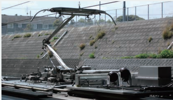
Rail vehicle fitted with the overhead contact line inspection system, Catenary Eye
