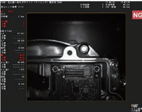
Image analysis of liquid gasket application
