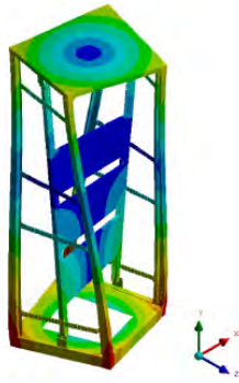
Structure analysis of switchboard
