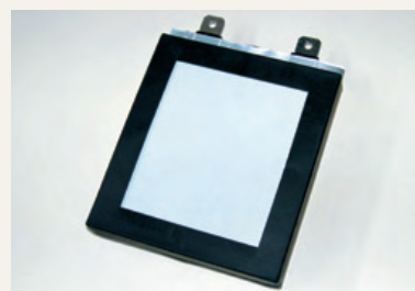
Image of electric double-layer capacitor (EDLC) using Aluminum-Celmet
