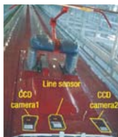
"Catenary Eye" (OCS inspection system)
