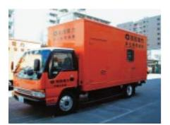
500kW Diesel Engine High-Voltage Generating System
