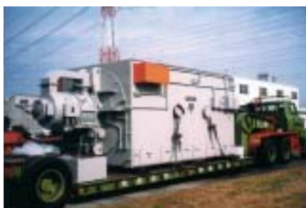
Gas turbine generator for GE LM6000PC
