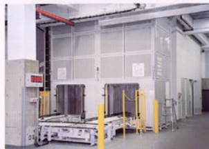
Vertical Carrier for Shipping Warehouse
